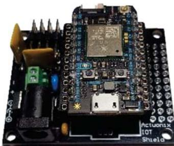
Photon Module installed
