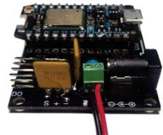
DC Power Supply Connected to +/-
